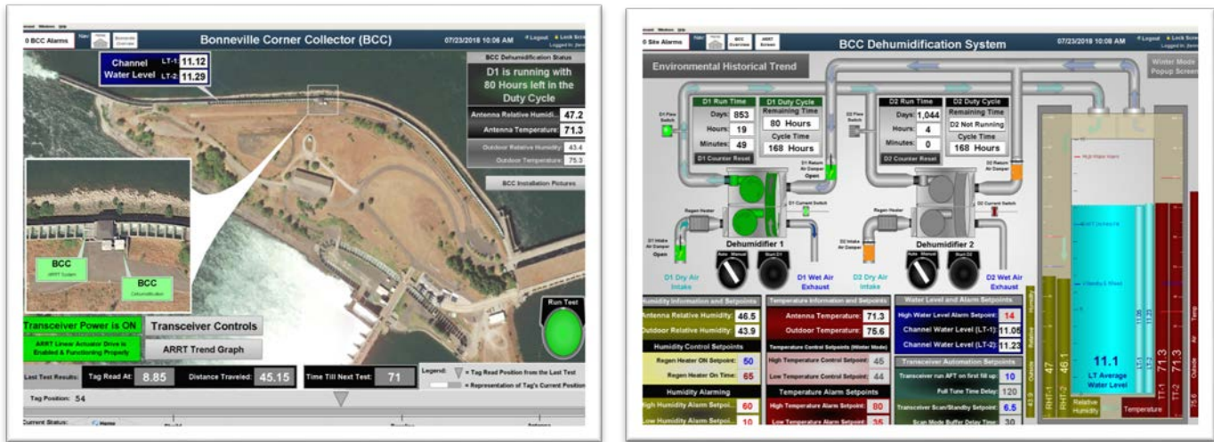
Figure 20. SCADA drill-through interface showing humidity-control automation for large antenna at Bonneville Corner Collector (BCC)
